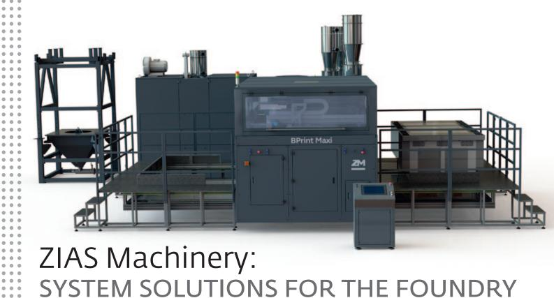
SINCE 2016 ZIAS MACHINERY HAS BEEN ACTIVELY DEVELOPING ADDITIVE TECHNOLOGIES IN THE FOUNDRY INDUSTRY. TODAY THE COMPANY IS THE ONLY RUSSIAN MANUFACTURER OF ZIAS BPRINT SERIES ADDITIVE UNITS FOR THE PRODUCTION OF FOUNDRY MOLDS AND CORES FROM SILICA SAND IMPREGNATED WITH FURAN BINDER.
